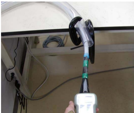
Fig.7 Simple insertion experiment using a dummy scope with force gauge
