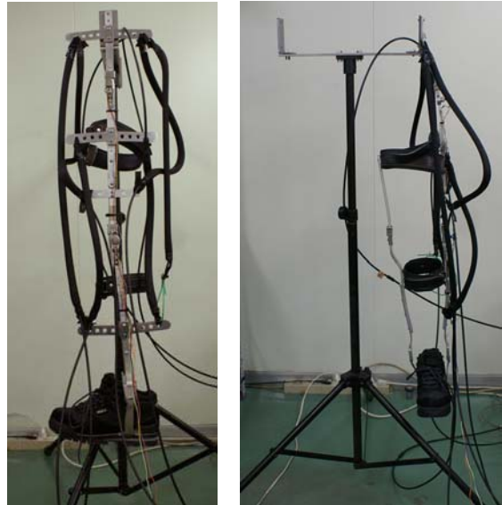
Figure 4 Left leg of orthosis
