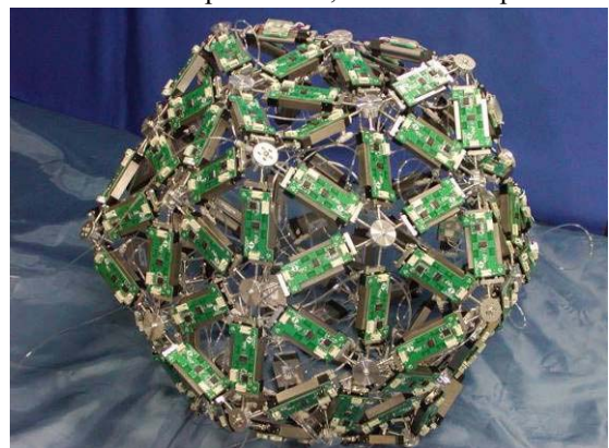
Fig.13 Active polyhedron consisting of 120 intelligent cylinders
