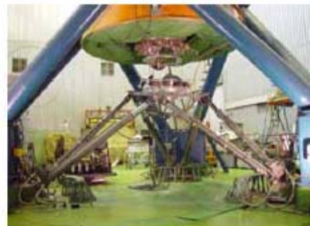
Figure1 Integrated testing system for docking mechanism
