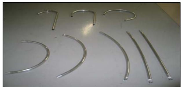
Figure 6 Results of the circular tube bending (aluminum)
