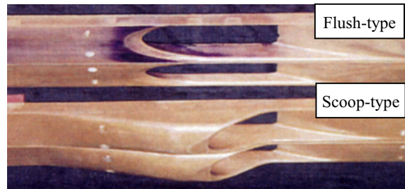
Figure 15 Model of the flush-type inlet (above) and scoop-type inlet (below)
