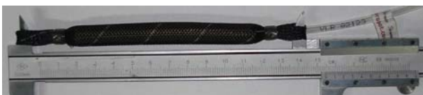
Figure 3 PMA of Shadow Company
