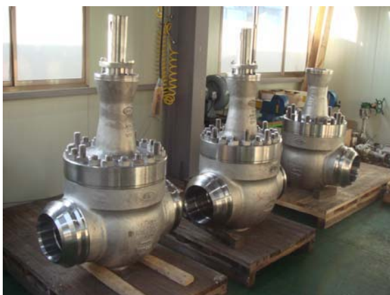
Figure 15 Cryogenic ball valve fabricated in this study
