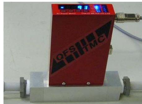
Figure .12 Photograph of air power meter
