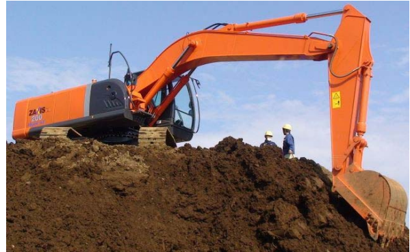
Figure 10 Picture of hybrid excavator
