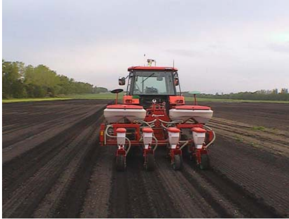
Figure 15 Planting soybeans by autonomous semi-crawler tractor (2007.5.29)
