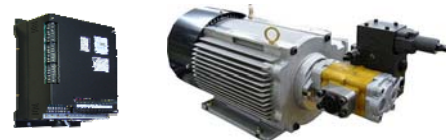
Figure 7 11 kW Super Unit for injection molding machines
