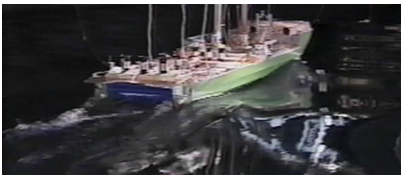
Figure 5 The model test in regular head sea
