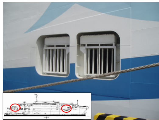
Figure 11 Photograph of the fore louver system
