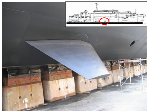
Figure 13 Photograph of the fin stabilizer system
