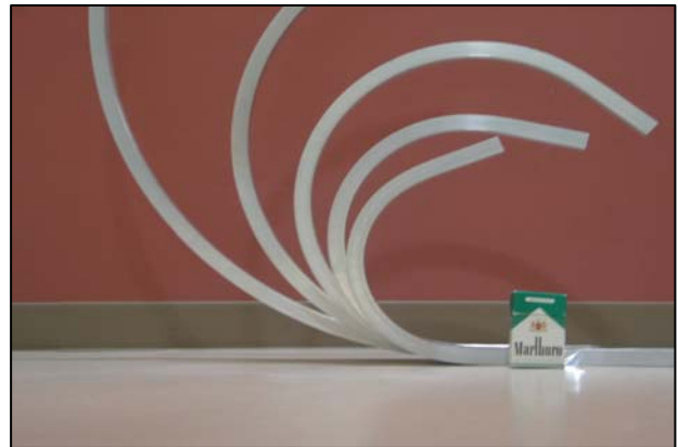
Figure 5 Results of the square tube bending (aluminum)
