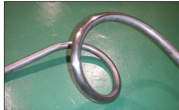
Figure 7 Result of the circular tube bending (steel)
