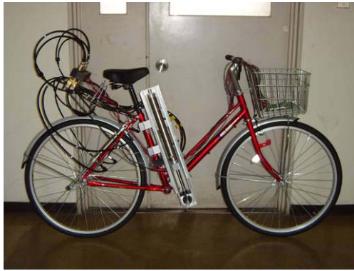
Fig.10 Prototype bicycle with pneumatic transmission
