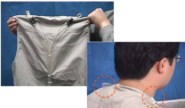
Figure 11 Wearable massage device mounting two pairs of FRT on the jacket
