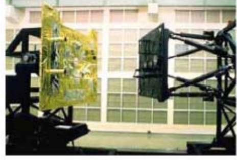
Figure 4 Rendezvous and docking operation test system
