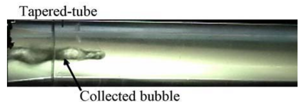
Figure 2 Flow visualization of trapped bubble
