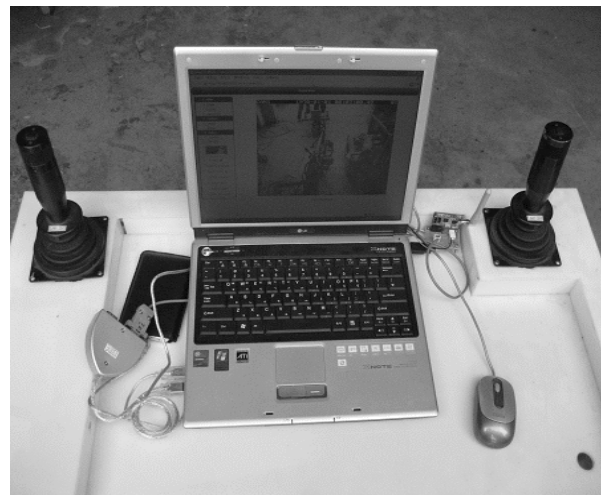
Figure 3 Remote operator station components
