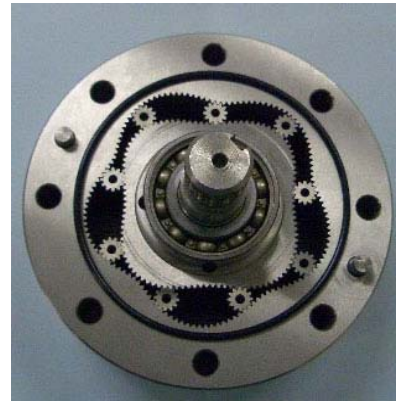
Figure 6 Inside view of the prototype of the water hydraulic planetary gear motor
