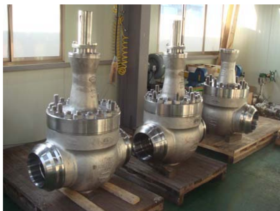
Figure 15 Cryogenic ball valve fabricated in this study
