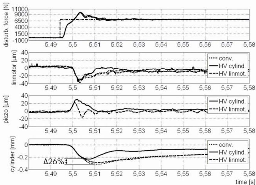
Figure 13 Disturbance rejection of the test cylinder
