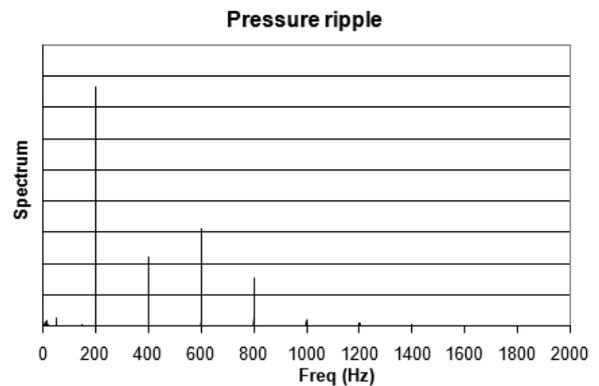
Figure 6 Pressure ripple (1000 rpm, 180 bar)
