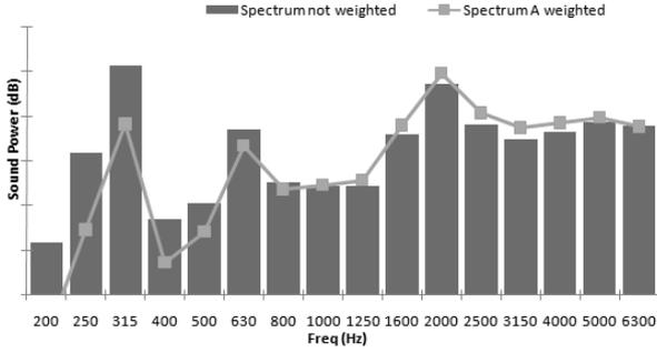
Figure 7 Sound power (1500 rpm, 180 bar)
