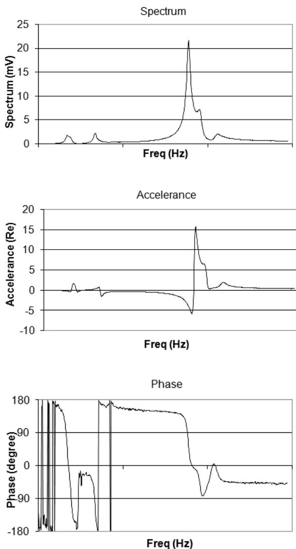
Figure 5 Harmonic transfer function: Spectrum, accelerance and phase vs frequency
