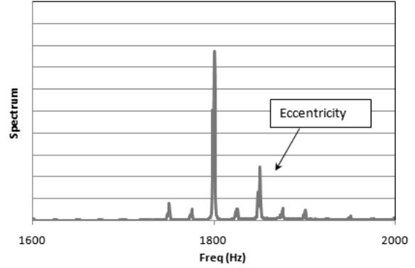
Figure 9 Spectrum of acceleration (1500 rpm, 180 bar)
