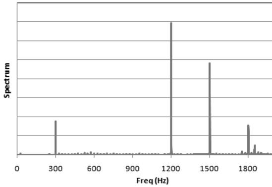
Figure 8 Spectrum of acceleration (1500 rpm, 180 bar)
