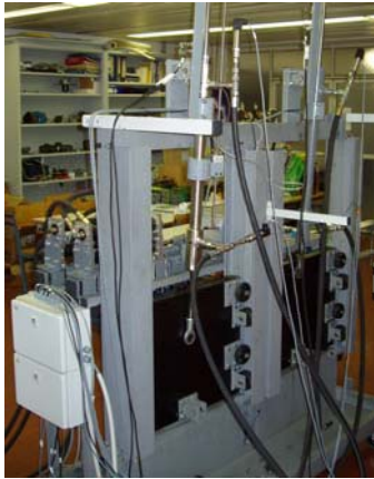
Figure 3 Water (on the left) and oil (on the right) hydraulic cylinder with load masses
