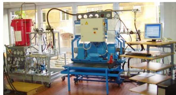
Figure 2 Water (on the left) / oil (on the right) power-control part of the test rig
