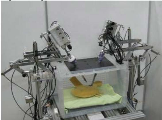
Figure.1 Developed slave manipulator
