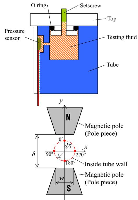
Figure 4 Schematic diagram and co-ordinate system of the experimental apparatus for measuring pressure
