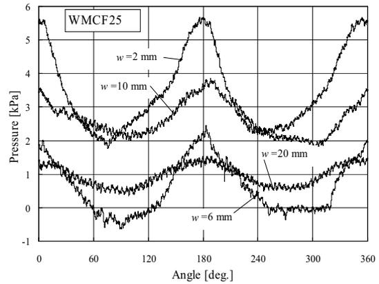
Figure 6 Pressure distribution inner tube wall (WMCF25)
