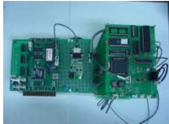
Figure 4 Image of the vehicle controller and the servo controller
