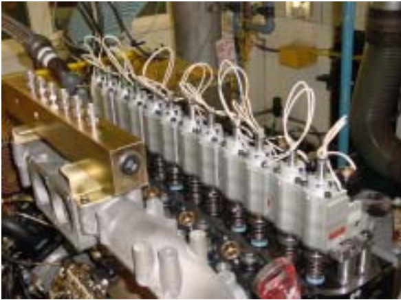
Photo 2 Valve actuators mounted on a 12L engine head
