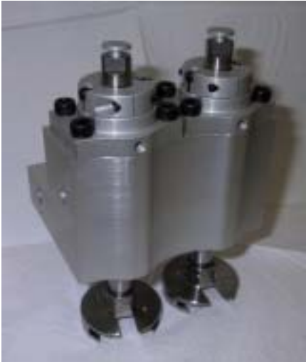
Photo.1 Electro-hydraulic valve actuator for gas exchange valve operated by high speed switching valves
