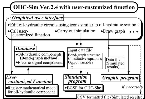
Figure 1 Basic structure of OHC-Sim
