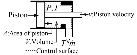
Figure 6 Rod-end chamber of pneumatic cylinder
