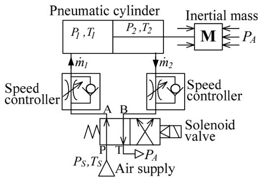
Figure 8 Pneumatic circuit
