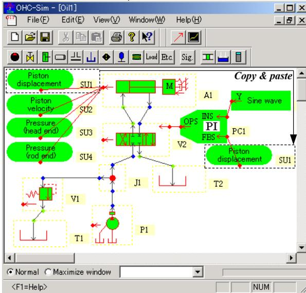
Figure 2 Edit of oil-hydraulic circuit by OHC-Sim
