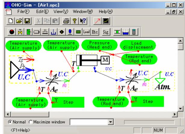
Figure 10 Edit of pneumatic circuit in OHC-Sim
