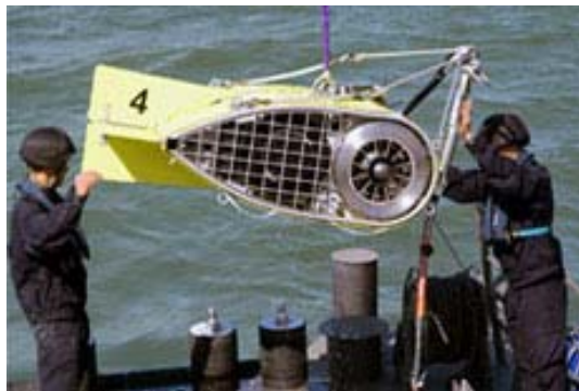
Figure 1. An example of magnetic hydro-sounder At low frequencies ( \leq 60 Hz) hydraulic hydro-sounder might be a reasonable solution. The principle idea of the hydraulic test system is shown in Fig.2.
