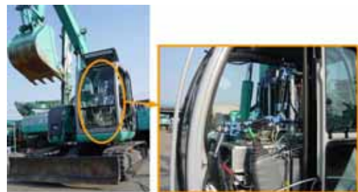
Figure 5 Developed remote control system installed in the operating room of the backhoe
