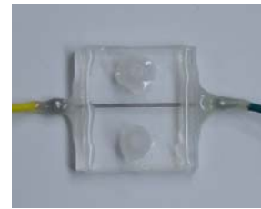
Figure 1 Top view of the EHD pump
