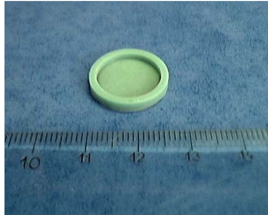
Figure 4. The silicone-based diaphragm
