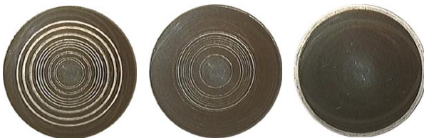
(a) E=0.5 kV/mm (b) E=1.0 kV/mm (c) E=2.0 kV/mm Fig. 11 Changes of ER fluid shear flow patterns with electric field strength ( t=300 sec, h=0.2 mm, AC50Hz)
