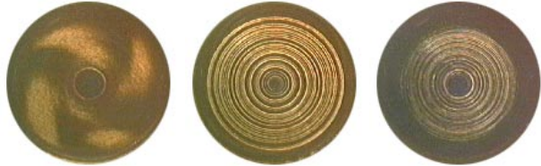
Fig.4 Changes of ER fluid shear flow patterns with electric field strength ( t=150 sec, h=0.2 mm, DC)
