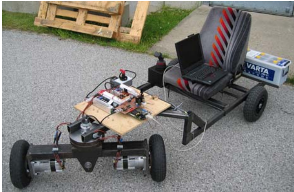
Figure 9 The prototype of designed and build vehicle with AC motor driven traction and steering
