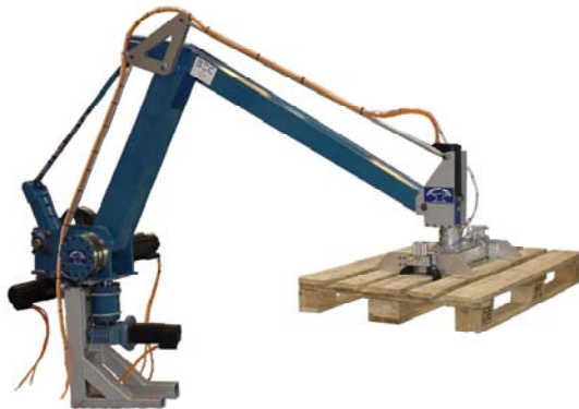
Figure 10 A 3 DOF servo robot for palette handling
