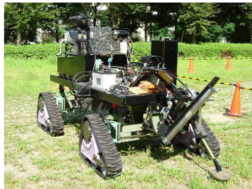
Figure 8 Robot applied in landmine field
