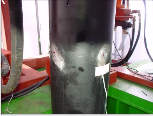
Figure 7 Strain gauge attached chisel
