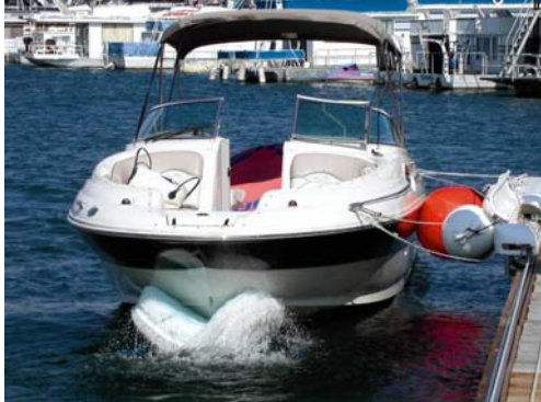
Figure 18 Automatic water hydraulic boat washer
