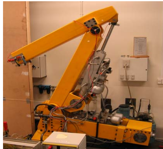
Figure 8 The DTU-AAU Hydraulic Test Robot
