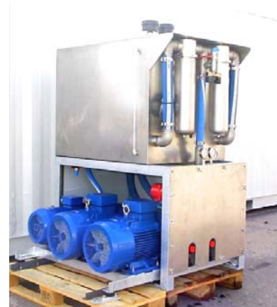
Figure 11 Water hydraulic drives for wing press equipment for an aero plane factory
