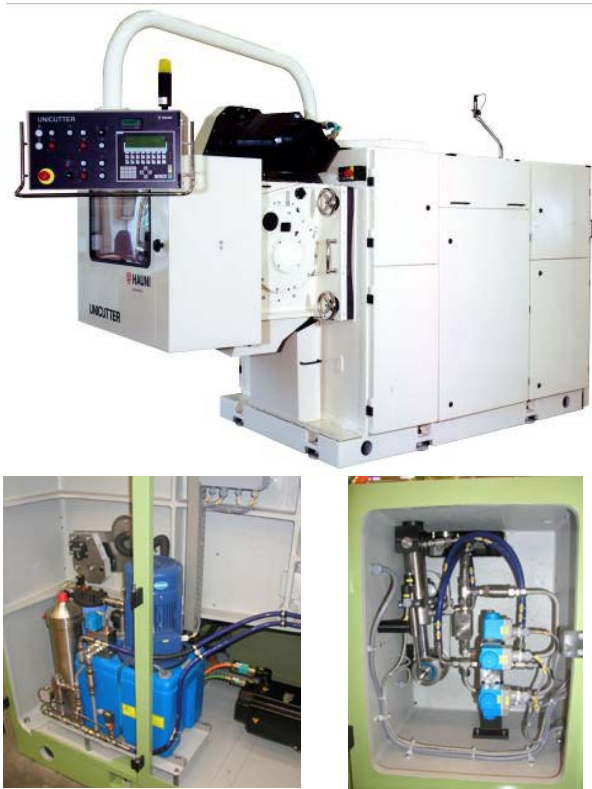
Figure 10 Automatic control tobacco cutter machine driven by water hydraulics with two cylinders
