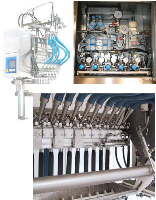
Figure 9 Ice fill machines for 400 ice per minutes with one motor, 3 linear servo cylinders and 3 end cylinders
