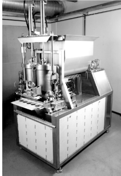
Figure 8 Tap water hydraulic driven burger-machine
