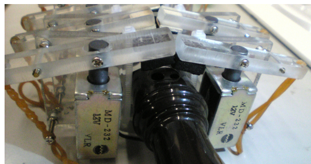
Fig. 2 Fingering part (solenoid plungers)
